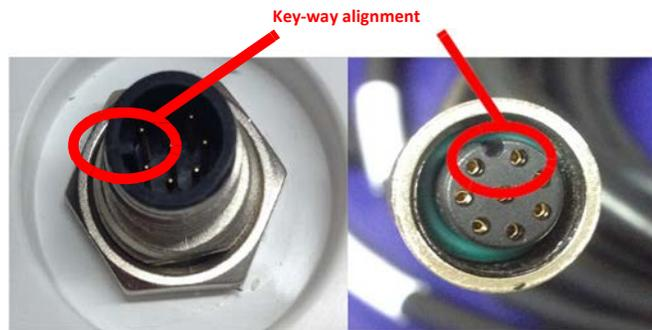
2. Rotate the cable ring clockwise until it locks. The locking action is firm, but you will feel a positive “click” when it has locked.
