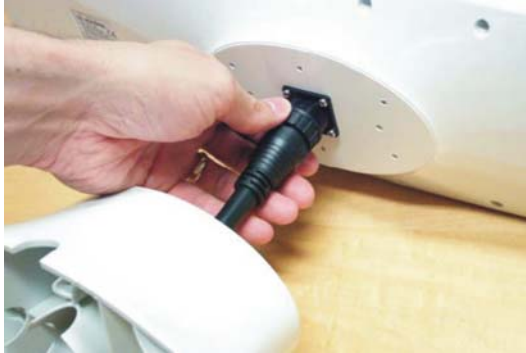
Figure 2-10: Connecting the power/data connector to V101/111
