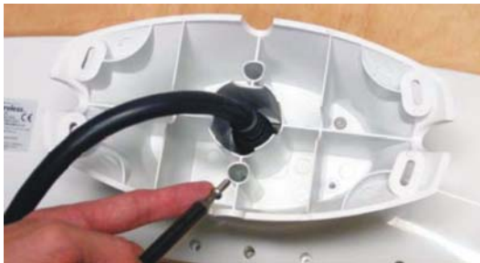
Figure 2-11: Fastening the fixed base to the V101/111
