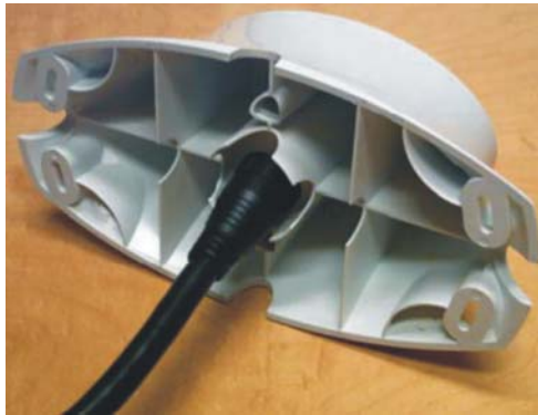
Figure 2-7: Running cable through fixed base mount
