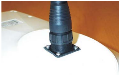
Figure 2-21: Connected power/data cable
