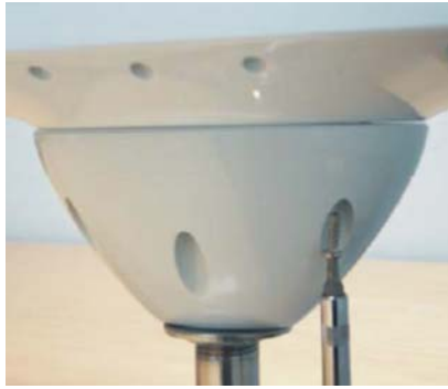
Figure 2-22: Fastening the pole base to the V101/111
