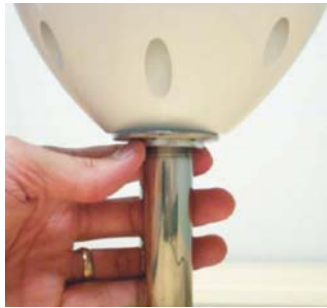
Figure 2-23: Threading the lock nut against the pole base
