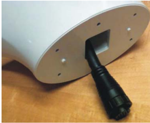
Figure 2-8: Running cable through fixed base
