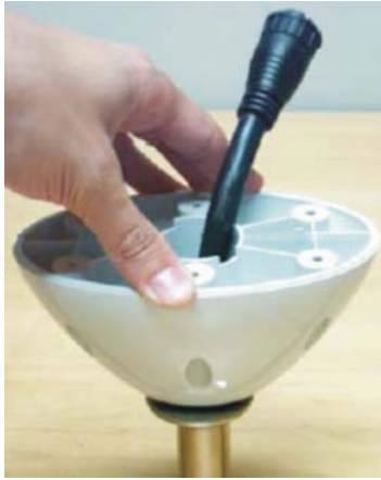
Figure 2-18: Threading the pole base onto the mount
