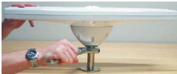
Figure 2-24: Locking the V101/111 once aligned
