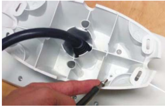
Figure 2-12: Fastening the fixed base to the V101/111
