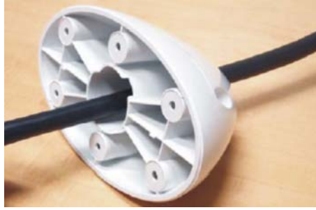
Figure 2-15: Running cable through the pole base
