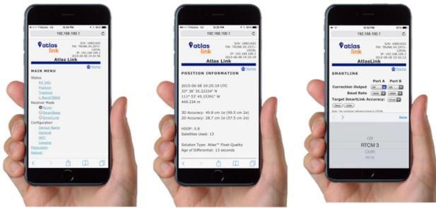
Figure 2 – AtlasLink web UI for configuring SmartLink
