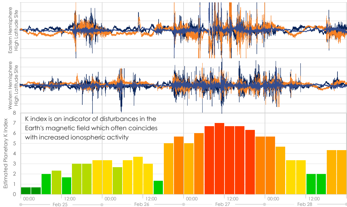
Figure 3: A measure of estimated ionospheric activity (bottom) compared to latitude, longitude, and height variations experienced at two high-latitude GNSS base station sites for the same timespan (middle and top). Estimated planetary K Index source: Space Weather Prediction Center, NOAA. https://www.swpc.noaa.gov/products/planetary-k-index © Hemisphere GNSS, 8515 E. Anderson Drive, Scottsdale, AZ, USA 85255 +1-480-348-6380 HGNSS.COM
